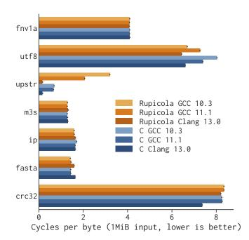
**Figure 2.** Performance benchmarks: Rupicola vs. handwritten C. Error bars indicate 95% confidence intervals for the mean over 1000 runs. Discrepancies are typically due to missed vectorization opportunities [39].
